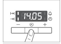
The function indicators Cook time → and End time → light up and the current time is shown in the display.
